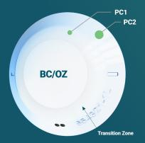
The Europa Tangent design incorporates a single curve scleral landing zone that is tangential to the average scleral curvature. With this design, the 5 curvatures that are present in the Europa Standard design are compounded into 3 parameters in the Europa Tangent design.
